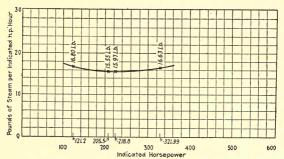
Fig. 266B.—Graph showing water rate of a 21 in. × 22 in. Skinner uniflow engine operating at a pressure of 149.1 lb. With a superheat of 102.5 deg. F.
